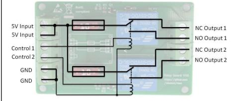
NC = normally closed (output connected if no control signal)
