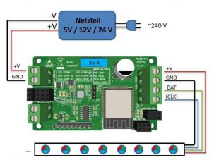
LED strip for example WS2812B / SK6812 / APA102 / WS2811 / WS2814
